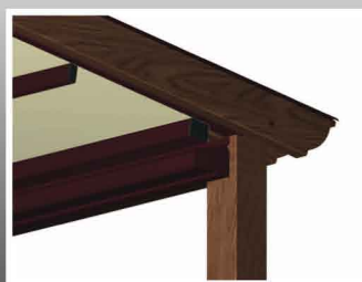
Gronda frontale Frontal water-drain
